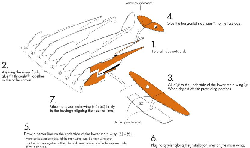
Placing a ruler along the installation lines on the main wing, make a dihedral angle of 8° for both sides of the main wing. (Use the dihedral angle gauge.)
